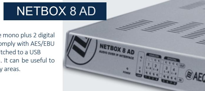
Provides 8 input and 8 output channels, distributed in 4 analogue mono plus 2 digital stereo connections. Stereo digital signals can be configured to comply with AES/EBU or SPDIF standards. The second digital stereo one can also be switched to a USB connector in order to facilitate the connection to a workstation. It can be useful to connect the console to recording cabins, booths or other auxiliary areas.
