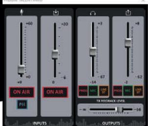
**CONTROL PHOENIX for TALENT** also incorporates an audio mixing screen, able to remotely adjust the level of the sound sources and select the signals to be sent to each output and its volume.
