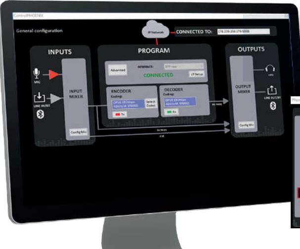
**CONTROL PHOENIX** allows for audio routing, communication mode selection, call establishment and level measurement and adjustment of incoming and outgoing audio signals for each audiocodec.
